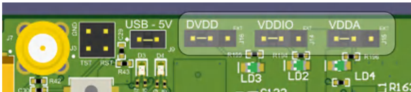
Figure 2-5. DP83TD510E External Supply Connection and Jumpers
