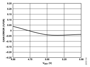
Figure 19. Gain Error vs. V<sub>DD1</sub>
