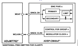
Figure 32. Interfacing the ADuM7702 to the ADSP-CM4xx
