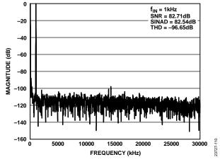
Figure 10. Typical Fast Fourier Transform (FFT)
