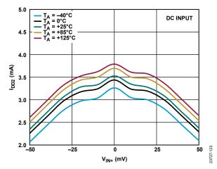
Figure 23. I<sub>DD2</sub> vs. V<sub>IN+</sub>, DC Input at Various Temperatures
