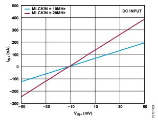
Figure 24. V<sub>IN+</sub> Current (I<sub>IN+</sub>) vs. V<sub>IN+</sub>, DC Input
