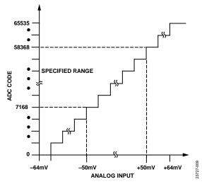
Figure 27. Filtered and Decimated 16-Bit Transfer Function
