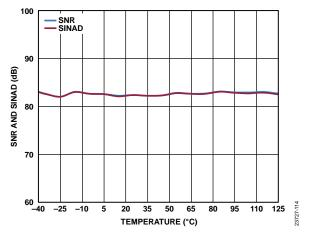
Figure 14. SNR and SINAD vs. Temperature
