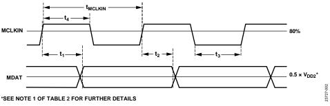
Figure 2. Data Timing Diagram
