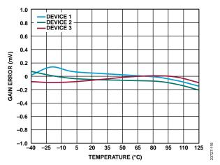
Figure 18. Gain Error vs. Temperature
