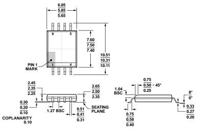
Figure 35. 8-Lead Standard Small Outline Package, with Increased Creepage [SOIC\_IC]
