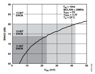
Figure 28. SINAD vs.  $V_{IN+}$  AC Input Signal Amplitude
