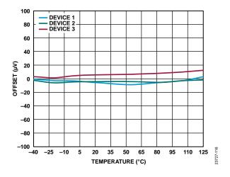
Figure 16. Offset vs. Temperature
