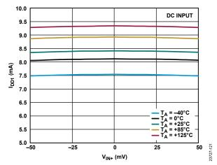
Figure 21. I<sub>DD1</sub> vs. V<sub>IN+</sub>, DC Input at Various Temperatures
