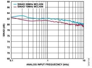
Figure 9. SINAD vs. Analog Input Frequency
