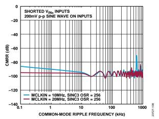
Figure 8. Common-Mode Rejection Ration (CMRR) vs. Common-Mode Ripple Frequency
