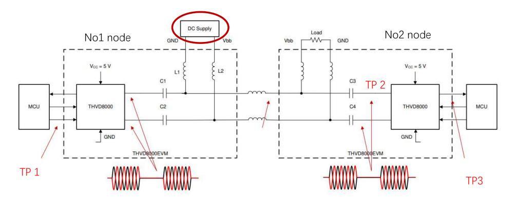
We used 3 powers, 1 is PC power(220VAC-20VDC), the PCBA was worked, TP2 and TP3 had signal. 2 is Adjustable switching power supply, TP2 had signal, the TP3 no signal , 3 is battery power , TP2 had signal , the TP3 no signal
