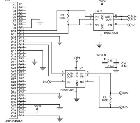
RX2+/RX2- and TX2+/TX2- lines must have differential impedance of 100 ohm with trace impedance of 50 ohm
