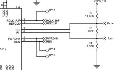
Resistors connected at the differential outputs of the Deserializer should be placed as close as possible to the Deserializer
