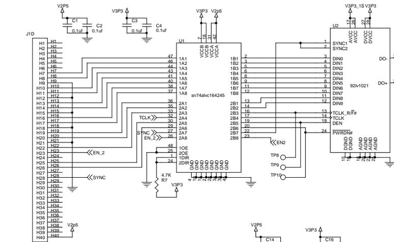
Resistors connected at the differential outputs of the serializer should be placed as close as possible to the serializer
