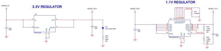
Figure 3. TUSB8020BPHPEVM Power Schematic
