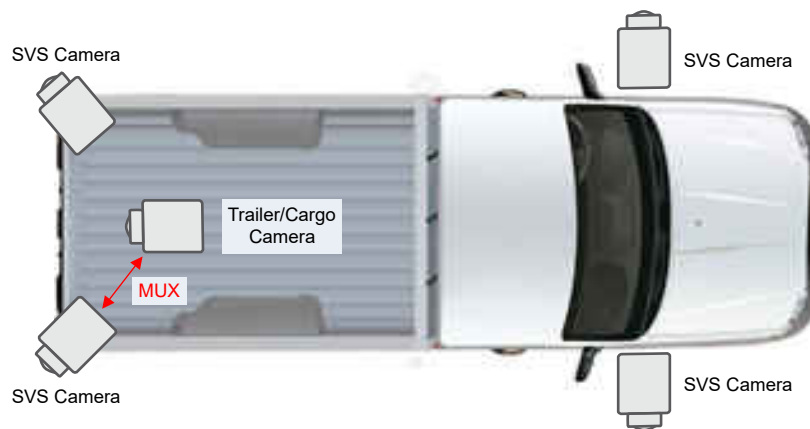
Figure 1-1. Automotive Application of Multiplexing FPD-Link SerDes
