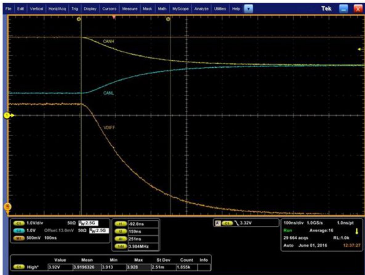
Figure 3. CAN Bus Signals with Only One Standard Termination (and One Missing)
