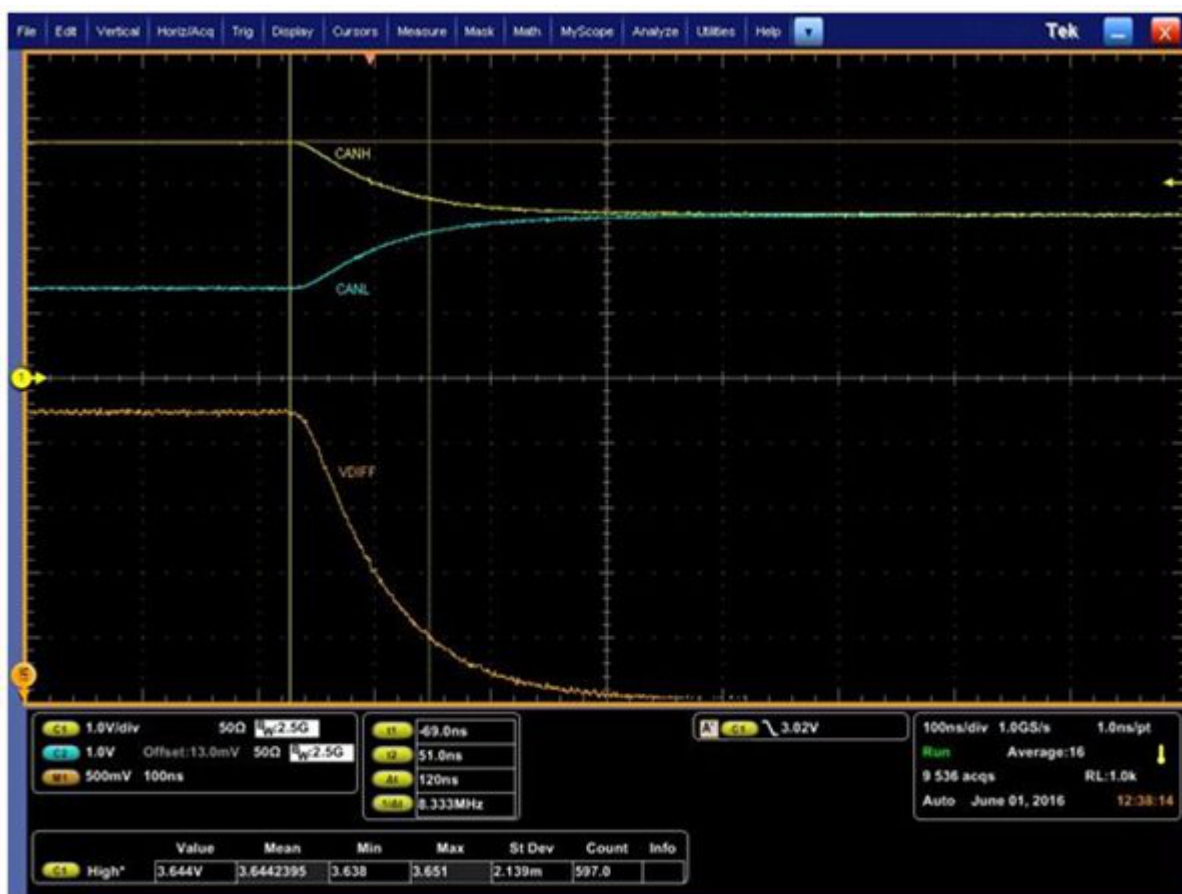
Figure 2. CAN Bus Signals with Two Standard Terminations
