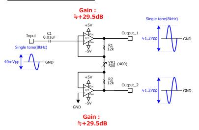
In the schematic above, if the input level is 40mVpp, is it possible that the output is about 1.2Vpp(about +29.5dB)?
