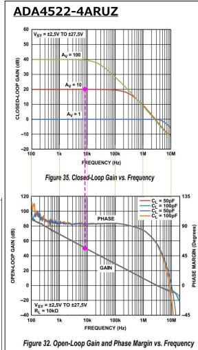
I am confused about the loop gain. In the schematic on the left, which is applicable, open loop gain or closed loop gain?
