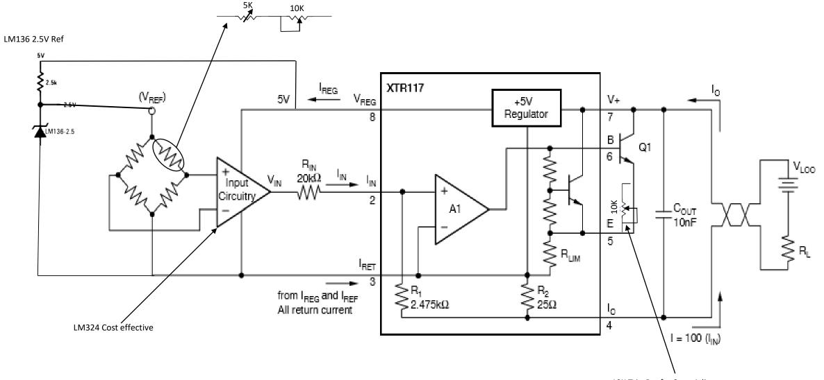
10K TrimPot for Span Adjustment
