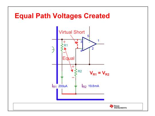
I mentioned that the voltage across R1 also appears across R2. This may not be intuitively obvious so here we take a closer look at this section of the circuit. The top of resistor R1 and R2 are connected together through the virtual short of the amplifier. The bottom of the resistors are connected at the lout line. The equal voltages in the parallel paths allow for the current to be scaled as needed.
