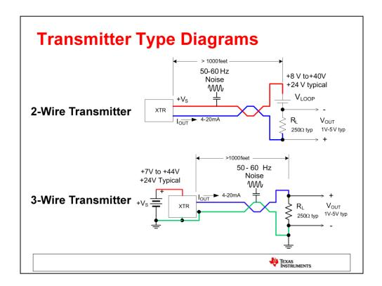
At this point we take a look at the basic diagrams of our transmitters. The two most common types of transmitters are the 2- and 3-wire types. As mentioned previously, an advantage of the current transmission line is immunity to noise, such as 50/60Hz power supply noise, that would otherwise couple into the long transmission lines.
