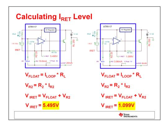
Why is it important to know what the current flowing through R2 is? To learn why the IRET pin can not be tied to ground we need to first determine what the voltage IRET reaches if left to float. The voltage level of IRET is calculated by the voltage created by the loop current flowing through the load resistor as well as the internal current flowing through R2. With a maximum-scale input of 160uA, for example, the voltage level of IRET is 5.495V.
