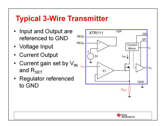
In contrast to the XTR117, the XTR111 has ground referenced on-board adjustable regulator that can be used to power external input circuitry. The regulator, though, does not necessarily *need* to be used to power the input circuitry since all voltages are referenced to the same GND. The current gain for this device is set with external components making it configurable to a variety of application requirements.
