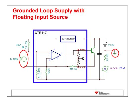
This is a simplified internal drawing of the XTR117. This circuit will allow us to see how the device operates and why it has the requirement of a floating input stage. One point to note about this circuit is the internal transistor section outlined in red - this section of the circuit is bypassed entirely when an external transistor is present so the internal transistor will be removed from further diagrams.
