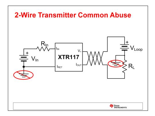
In starting to look into the operation of the circuit, I'll first show this diagram. This XTR117 circuit can not operate correctly because the input is referenced to the same potential as the loop supply which violates the predefined operating conditions of the XTR117. The input circuitry and IRET must be allowed to float with respect to the loop supply ground. With IRET pin pulled to ground, the IRET pin can not float to the necessary voltage required to allow for the circuit to work properly.
