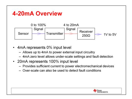
The typical 4-20mA transmission path is shown here, starting with the sensor on the left. The sensor measures a variable over a specific range, for example, a temperature between 0 and 500°C, and outputs a signal proportional to where the measurement falls within the set range.
