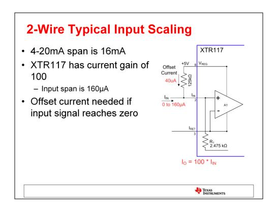
Here we see the input side of the 2-wire current transmitter XTR117. This device generates a current output proportional the current received at its input.
