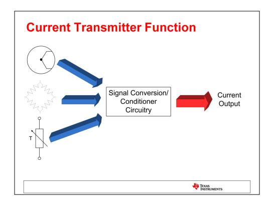
Let's now look a little more closely at the function our XTR current transmitter parts perform. Transmitters are frequently used to send a proportional signal generated from a sensor measuring a real-world parameter, to a receiver which is typically located at a distant location. Our XTR current transmitters allow us to perform this task, as well as condition the signal depending upon the sensor's inherent properties.
