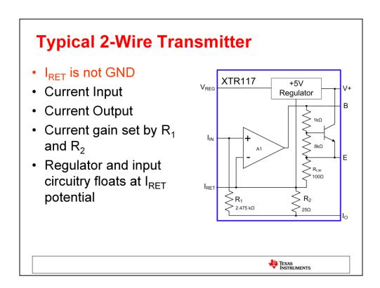
To further break down the differences in how these 2 and 3-wire transmitters are different, we need to look into how the 2-wire internal circuitry operates. To highlight one of the main aspects of the two-wire transmitter, the IRET pin is not GND. We will soon see why this is such an important condition for the proper operation of this device.
