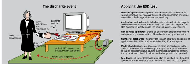
normal operation; not necessarily pins of open connectors nor points accessible only during maintenance or servicing used where contact cannot be applied; both direct discharges to the EUT, and indirect discharges to the coupling plane(s), are required Number of discharges- normally ten in each polarity to each point of plication – EN 55024 requires a total of 200, 50 at each point urface of the EUT; for air discharge, the tip must approach the EU
