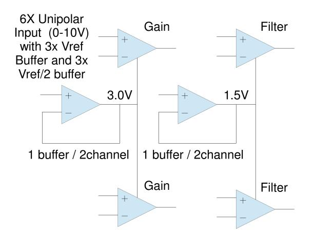
All ADC channel have the same configuration except for the gain resistors and the input offset voltage.
