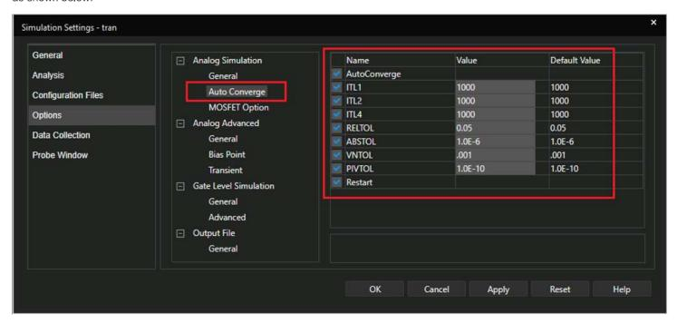
You could activate the AutoConverge option and run the simulation. Above functionality should avoid your most of the convergence problem but below are few troubleshooting guidelines for Convergence Failure:
