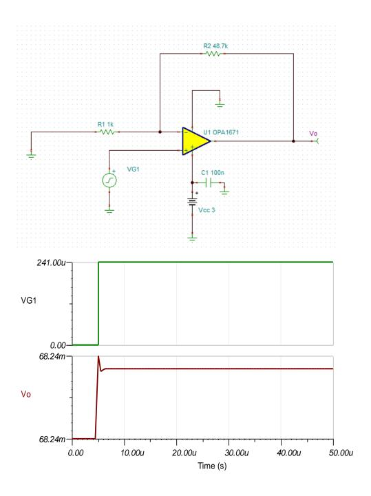
This is the circuit used for indirect phase margin measurement
