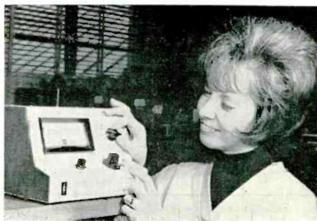
Engineering-laboratory test set for measuring unijunction transistor's characteristics. This instrument whose circuitry contains unijunction transistors, measures seven characteristics including intrinsic standoff ratio and interbase resistance. It is manufactured by the Syracuse Electronics Corp.
