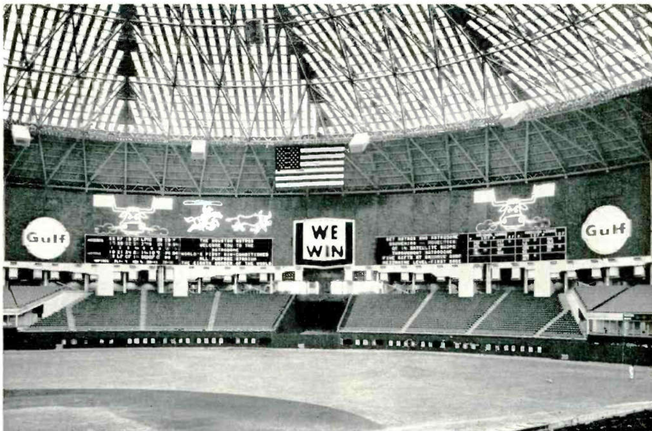
Scoreboard at Astro-dome Stadium contains nearly 200,000 semiconductor devices including about 25,000 unijunction transistors. The center section of the scoreboard, showing the message "we win," can also display scenes and pictures of players. The manufacturer is the Fair Play Scoreboard Co.
