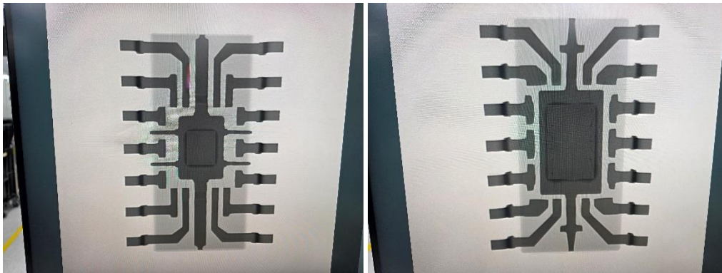
Picture 2: X-Ray pictures of TLC274C Passed the test date code 101000000076609 in the left side and Failed the test date code 101000001170243 in the right side.
