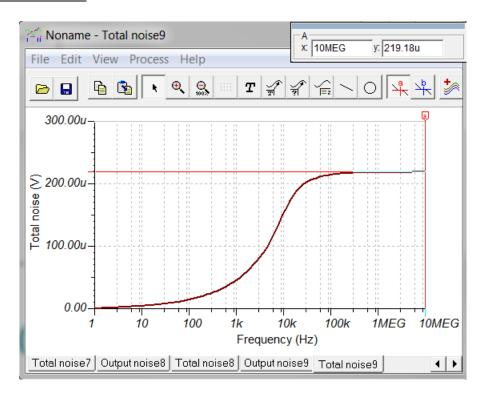
Simulation Total noise =  $219.18 \mu V_{RMS}$ Hand Calculation Total noise =  $211.76 \mu V_{RMS}$
