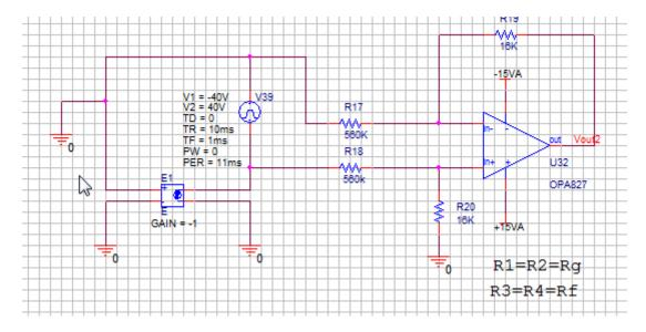
ERROR(ORPSIM-15143): Voltage source and/or inductor loop involving V\_V39. You may break the loop by adding a series resistance
