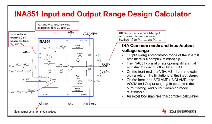
Instrumentation amplifiers are composed of multiple op amps. This figure shows the simplified INA851 configuration. Each amplifier inside the INA has it's own input and output swing limitations. These limitations combine into an overall common mode versus output swing range limitation for the instrumentation amplifier.
