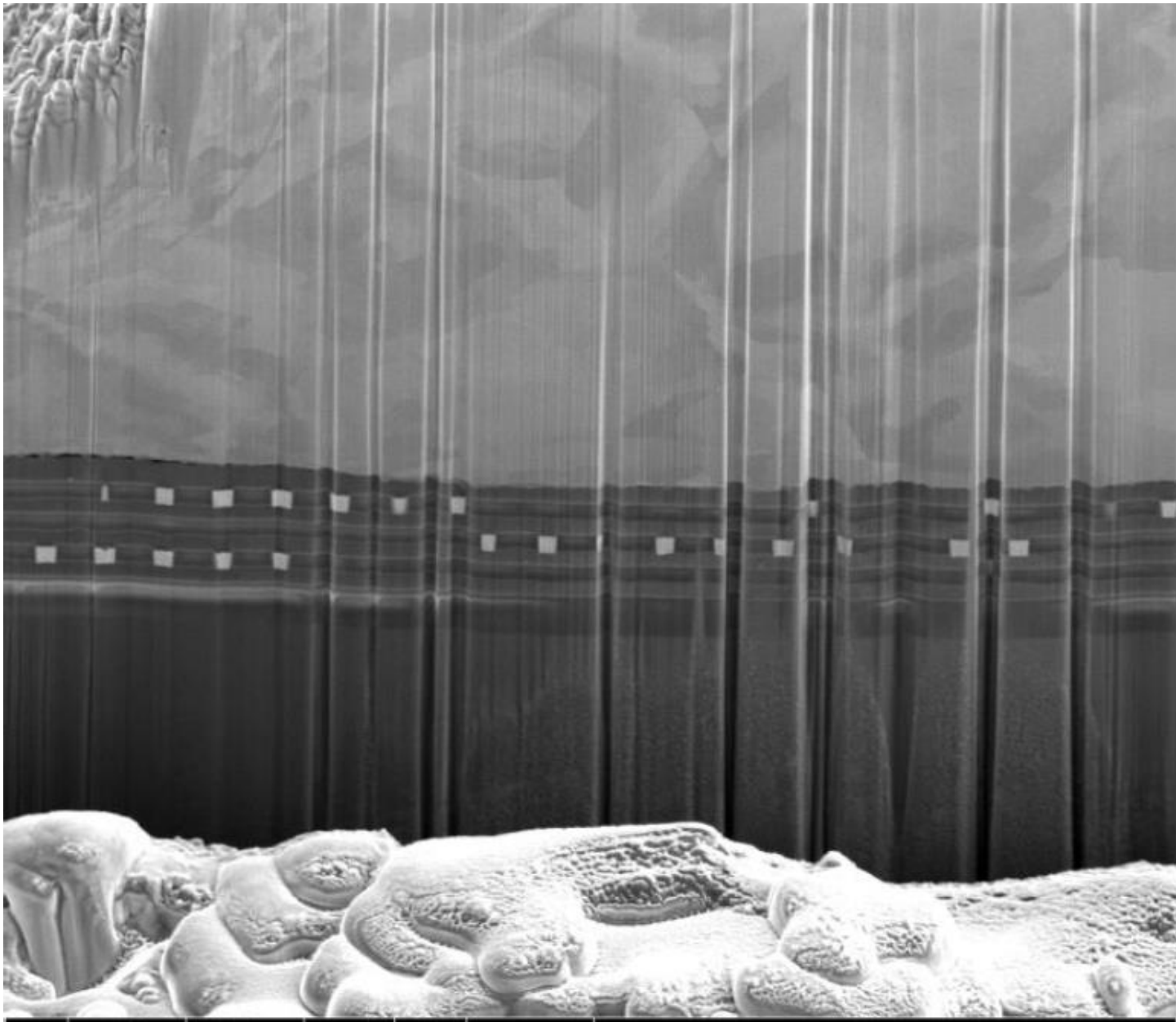
Zoom in the cross-section of unit #2. Inner bonding layers are not damaged.
