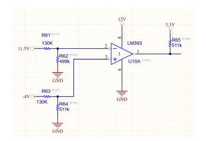
In the above circuit, LM393 pin 3 sits at -0.49V. Will that damage LM393? Current out of pin 3 = (-0.49V + 4V)/130kohm = 19.3uA.
