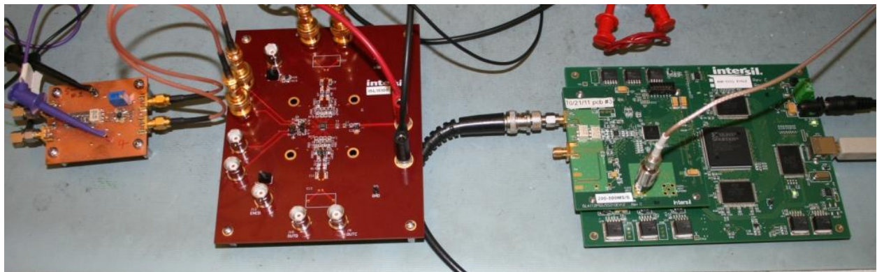
Figure 2. Test hardware for PLC line driver MTPR evaluation
