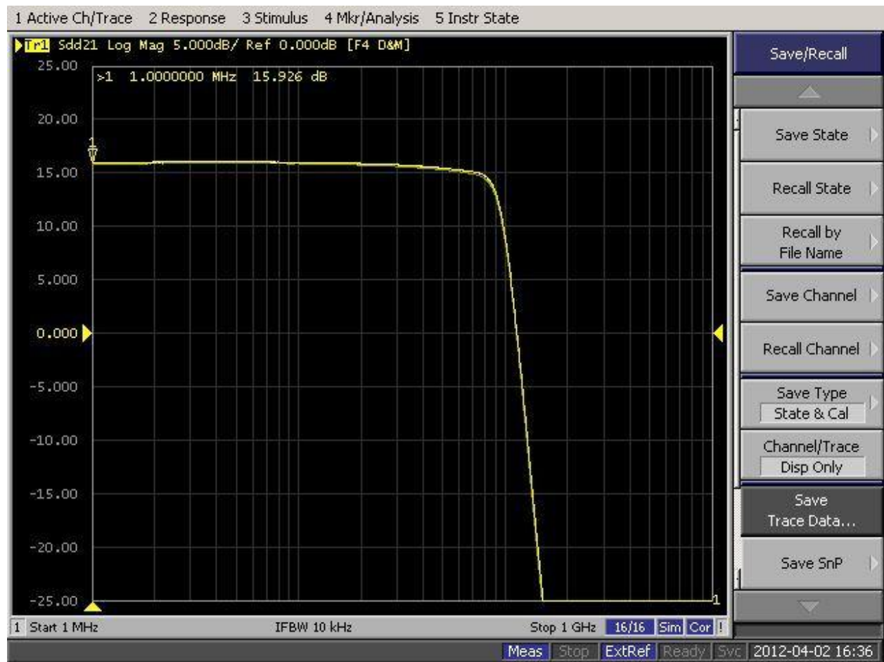
Figure 4. Broadband response magnitude sweep for ISL55210 based AWG postamplifier.
