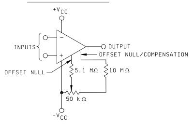
FIGURE 2. Offset null circuits.
