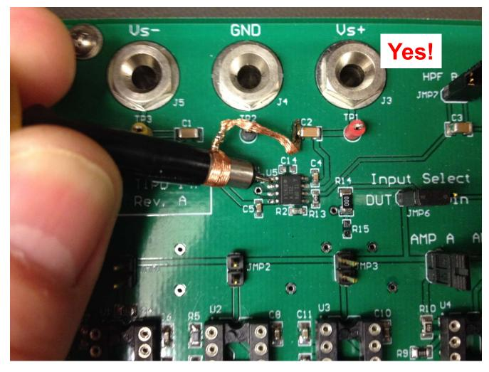
Connect tip of scope probe directly to point to be measured. Solder "solder wick ground" very, very close to IC ground
