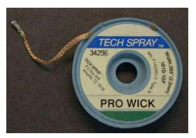
Desoldering braid, also known as desoldering **wick** or **solder wick**, is finely braided 18 to 42 AWG copper wire coated with rosin flux, usually supplied on a roll. The end of a length of braid is placed over the soldered connections of a component being removed.
