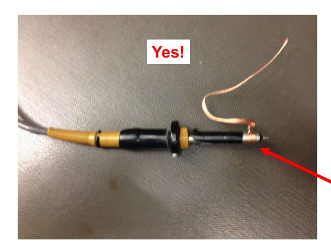
Use solder wick for a good high frequency ground connection.
