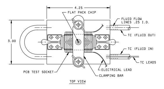
FIGURE 1012-1. <u>Temperature controlled heat sink</u>.
