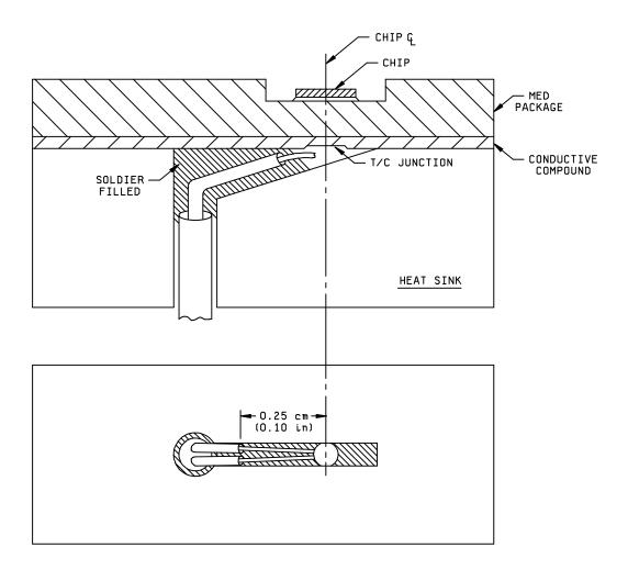
FIGURE 1012-2. <u>Temperature arrangement for mounting surface temperature measurements</u>.
