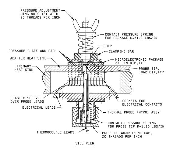
FIGURE 1012-1. Temperature controlled heat sink - Continued.
