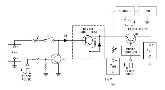
FIGURE 1012-4. Typical test circuit for indirect measurement of  $T_{J(Region)}$  using the substrate diode of junction isolated integrated circuit.
