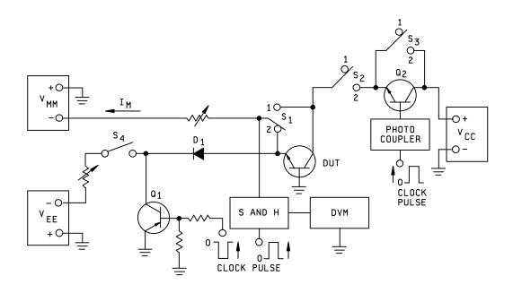
TSP: Diode  $V_F$  - Switch S1 in position 2
