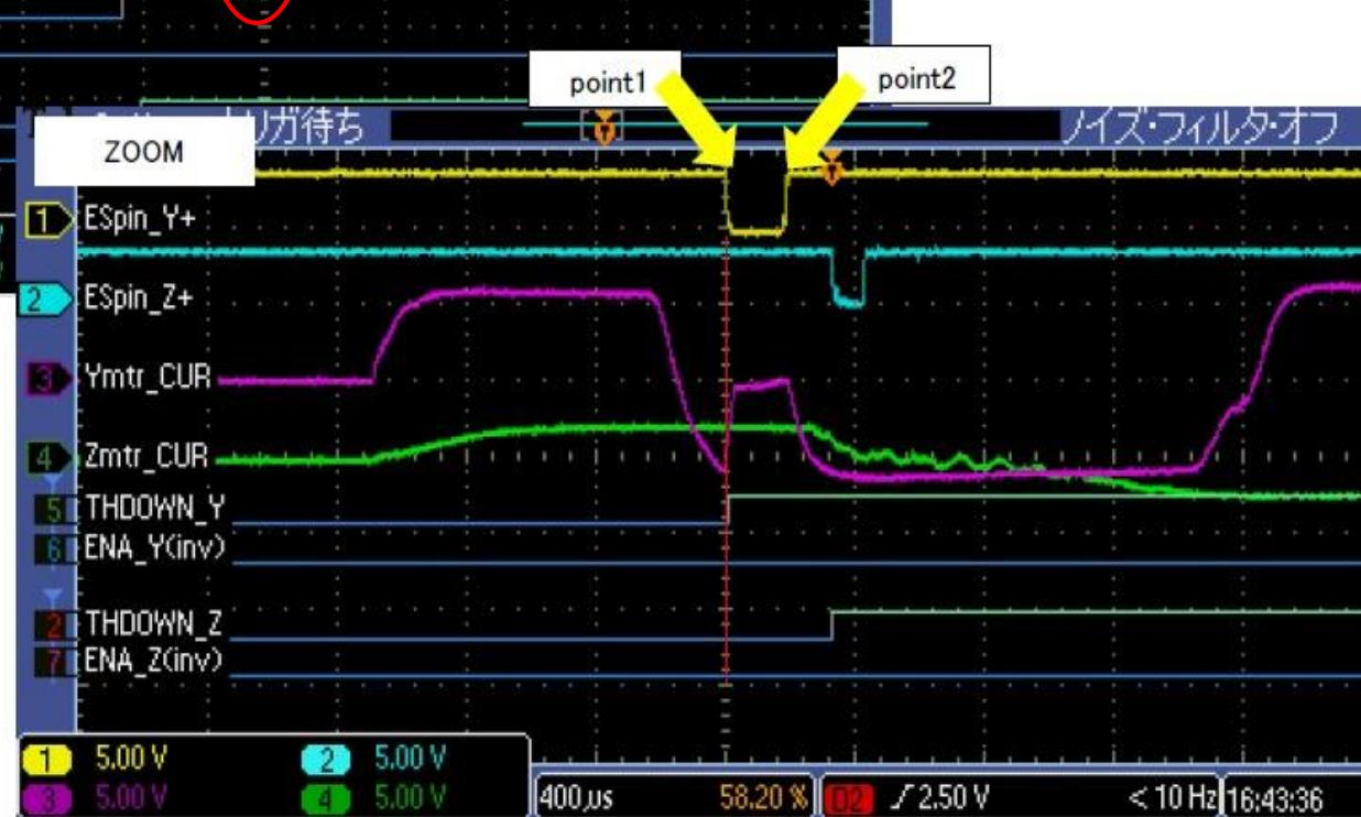
This is the waveform of Thermal Shutdown Status (E / S pin) observed. Please see only ch1 and ch3.
