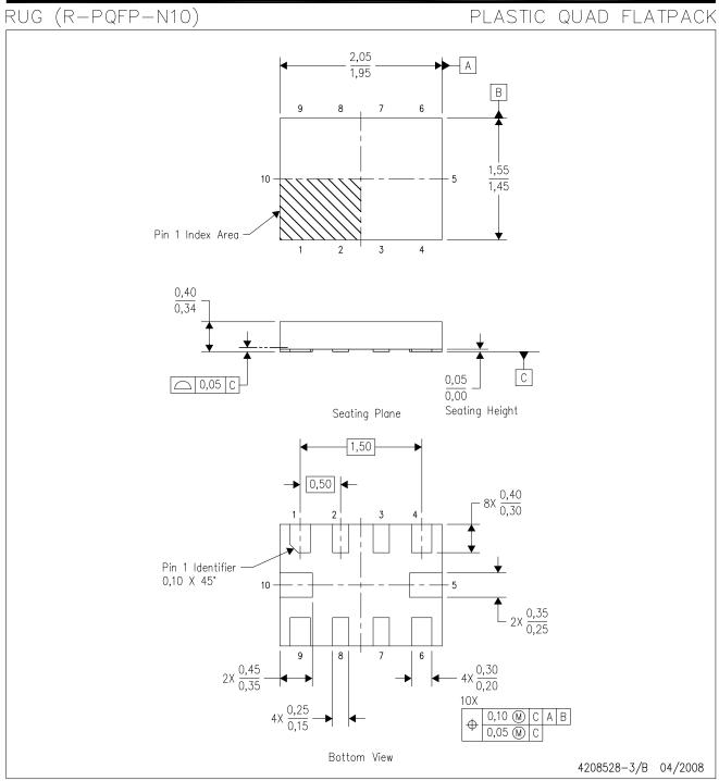
NOTES: All linear dimensions are in millimeters. Dimensioning and tolerancing per ASME Y14.5M-1994.
