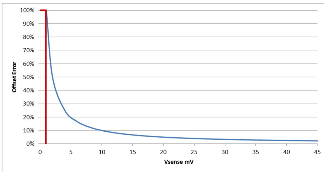
$$\text{Offset Error} = \frac{1 \text{ mV}}{1 \text{ mV}} * 100 = 100 \%$$
