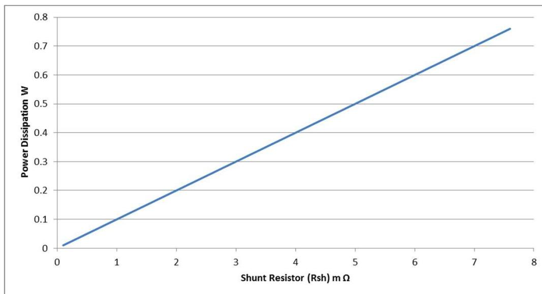
$$\text{Power Dissipation} = R_{sh} * I_{load}^2$$
