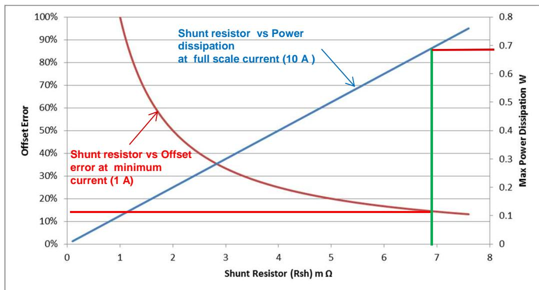
$$\text{Offset Error (in percent)} = \frac{1 \text{ mV}}{6.66 \text{ mΩ} * 1 \text{ A}} * 100 = 15 \%$$
