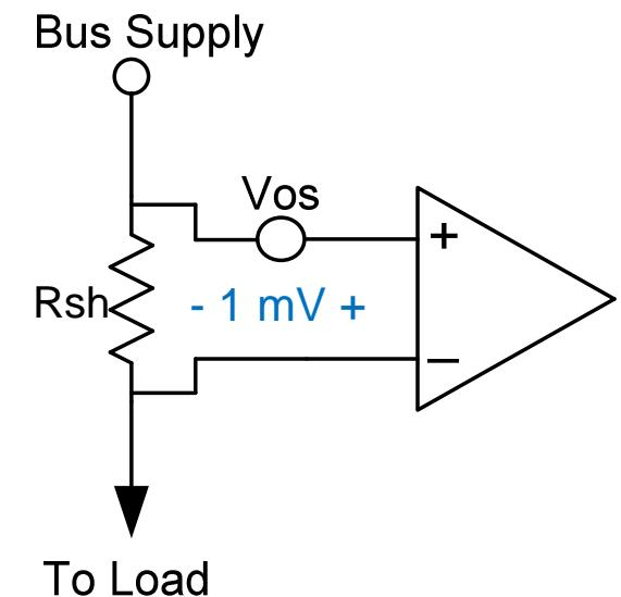
$$\text{Offset Error (in percent)} = \frac{V_{os}}{R_{sh} * I_{load\_min}} * 100$$
