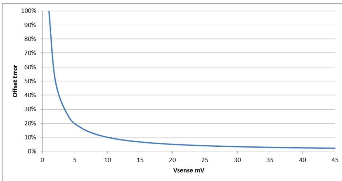
$$\text{Offset Error (in percent)} = \left( \frac{V_{os}}{V_{sense}} \right) * 100$$
