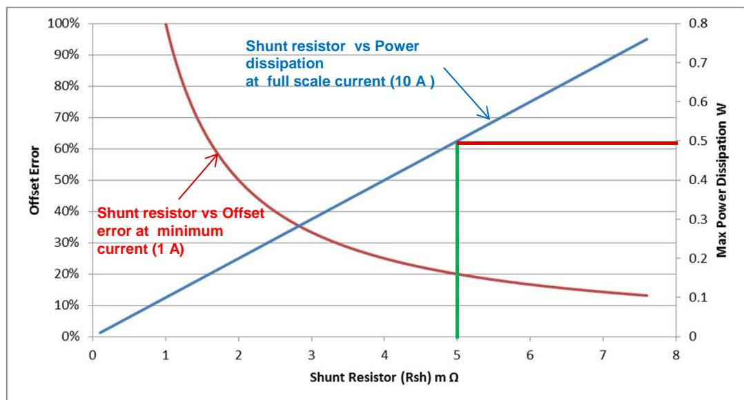
$$\text{Offset Error (in percent)} = \frac{1 \text{ mV}}{5 \text{ m}\Omega * 1 \text{ A}} * 100 = 20 \%$$
