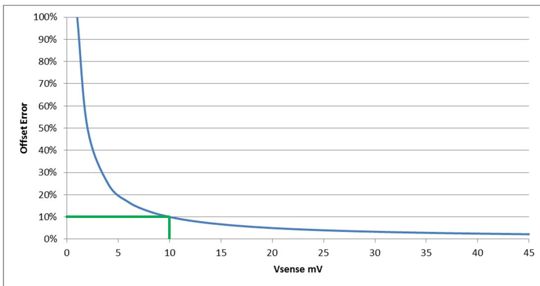
$$\text{Offset Error} = \frac{1 \text{ mV}}{10 \text{ mV}} * 100 = 10 \%$$
