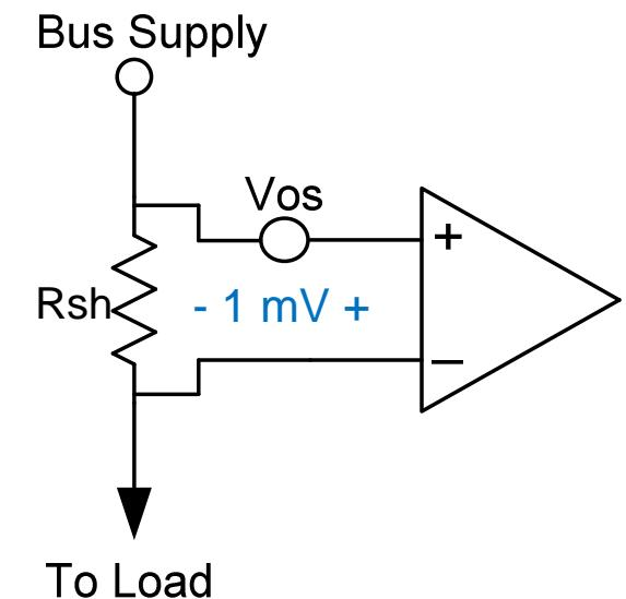
I<sub>load\_min</sub> = 1 A; I<sub>load\_max</sub> = 10 A
