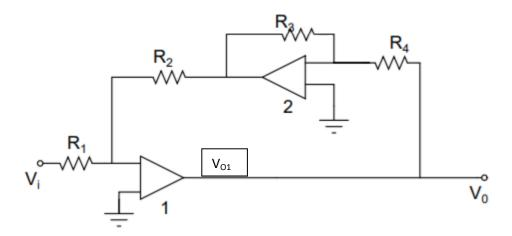
Let the O/P of A1= $V_{01}$ then the O/P of A2=(R4/R3) $V_{01}$
