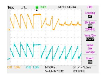
Video buffer (op-amp input) has significant overshoot/undershoot (ringing) due to high BW and fast edge rates.
