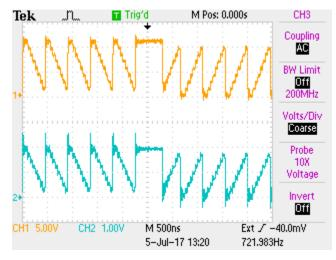
Just to illustrate the desired input signal – provided by a high-speed D/A converter running at 25 Msps (goal). This test image generates an 8-step ramp between #00 an #FF values before repeating.
