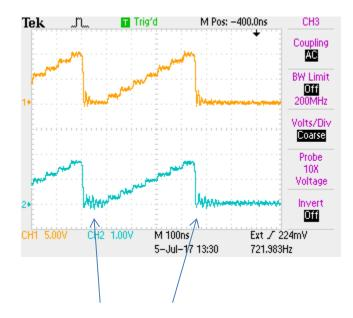
Close-up of undesirable video buffer ringing, although this opamp doesn't seem to have a problem with it.
