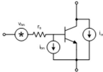
**Fig. 7.6: Bipolar Transistor Noise Model**
