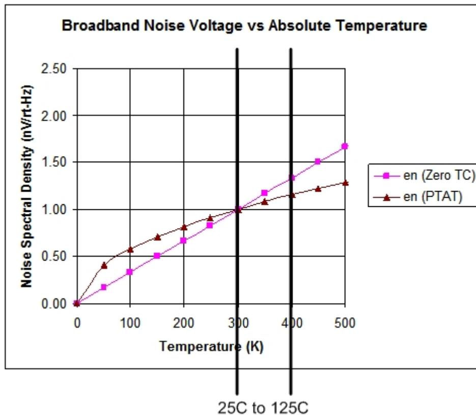
**Fig. 7.2: Worst Case And Typical Variations Of Noise Vs Temperature**
