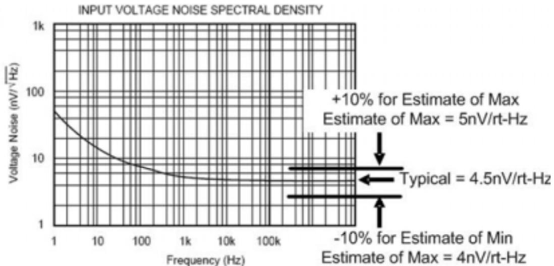
Fig. 7.1: Estimate Max Room Temperature Broadband Noise Based on Typical
