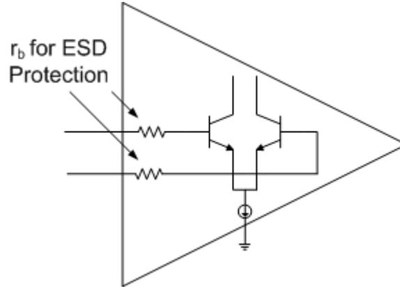
**Fig. 7.8: Thermal Noise Component Of Op Amp Noise**
