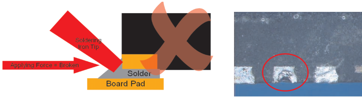
Figure 18. Manual Rework Damage
