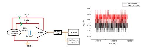
Now I running the setup (I think same as you suggested?) see below. I can see the output of the EO and the op-amp are the same but different than the output of the separated EO, you can see the frequency is now 5.875 MHz which is different than the 5.74 MHz of the separated EO. beside the output amplitude of EO is different than the separated EO.
