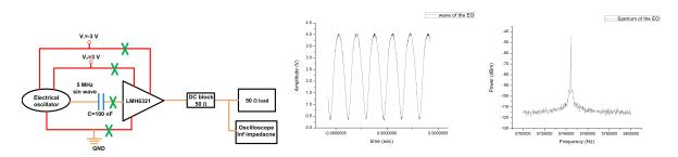
We can see that the EO output an almost sin wave with frequency of 5.74 MHz.
