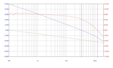
Figure 10.1 Loop Bode Plot (Vin=3.6V, Rload=6 ohm)
