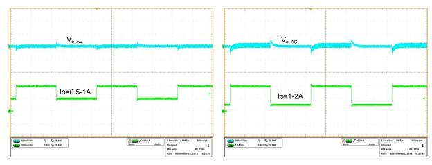
Figure 9.1 and Figure 9.2 show the load transient response of the output voltage.
