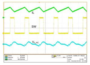
Figure 7.1 Switching Waveforms at Vaudio=0V
