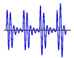
Figure 1. Audio Signal with High Peak to Average Ratio
