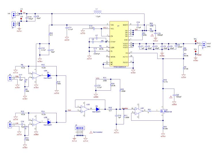
Figure 11. Schematic of the Reference Design with LMV324
