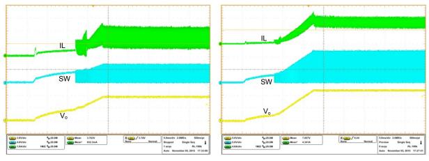
Figure 8.1 Startup Waveforms at Vaudio=0V
