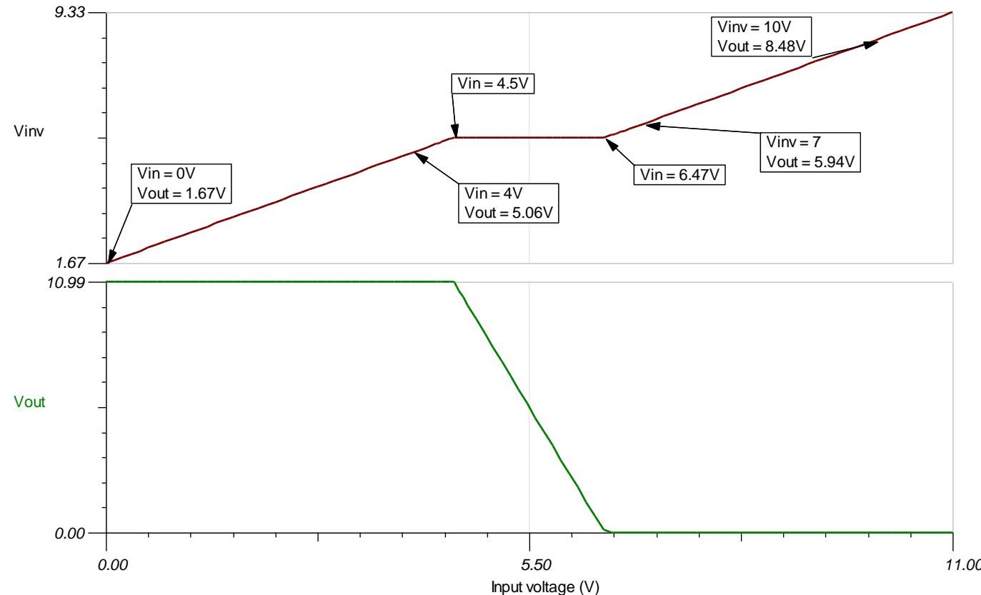
Below 4.5V and above 6.47V the circuit is open loop. To understand  $V_{inv}$  in this case you can just erase the op amp and think of this as a series circuit with two power supplies:  $V_{out}$  and  $V_{in}$ . The equations in these two regions are given to the right.
