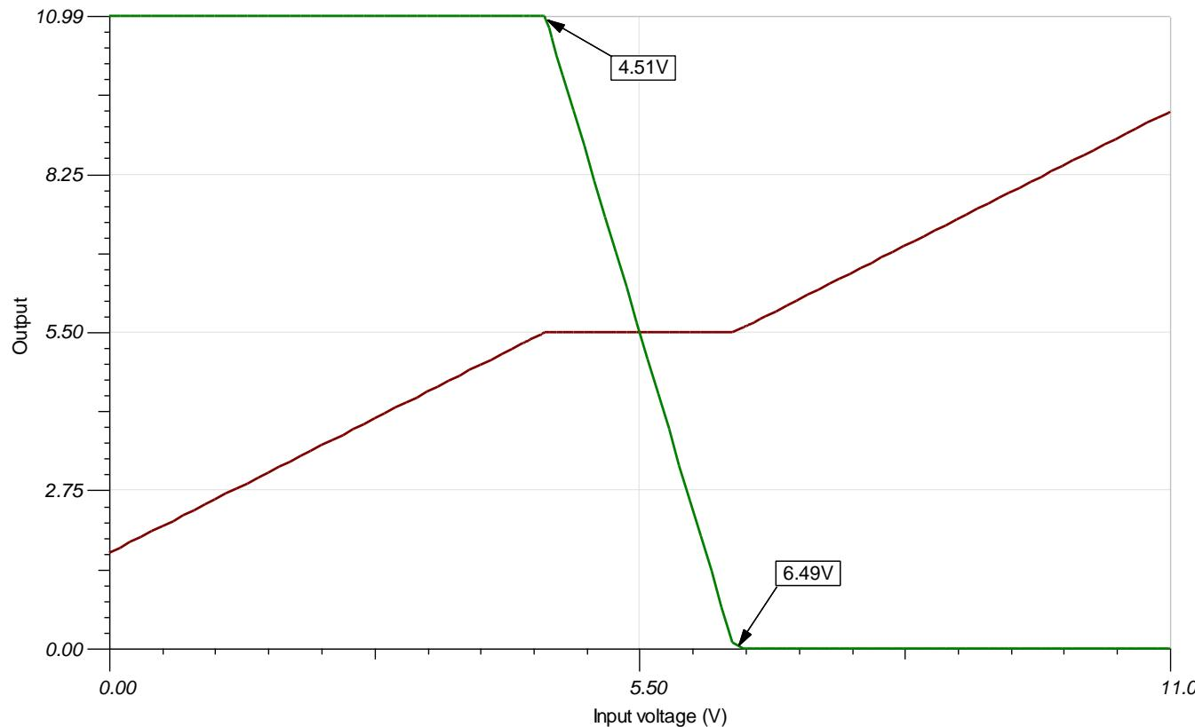
Here is the circuit without the diodes. Note that the output is only linear for input signals from the range of 4.51V to 6.49V. This is predicted with both simulation and calculation
