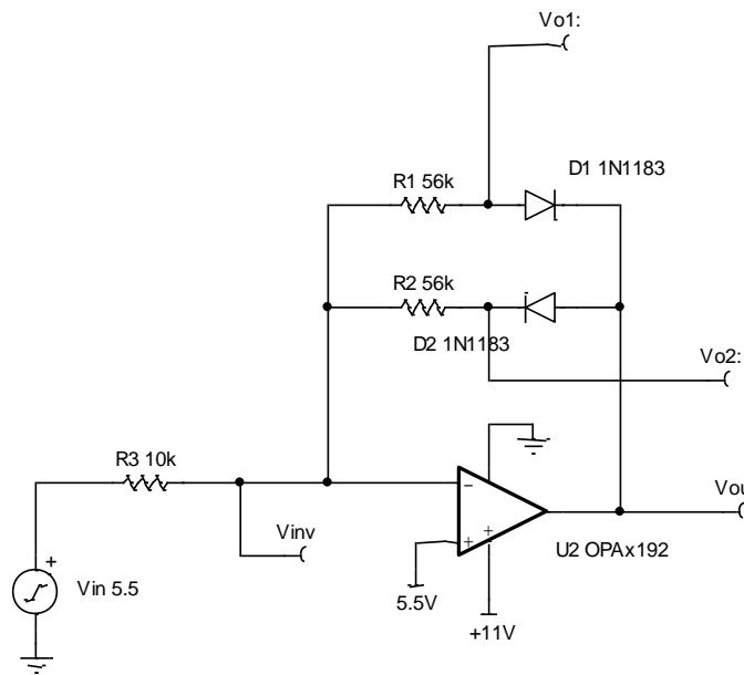
Add the diodes back in and look at the output pin. Notice from the output pin perspective, the two circuits are basically the same. If you look closely at the circuit with diodes you will see a small non-linearity when the output signal passes through 5.5V. The non-linearity occurs when switching from one diode to the other diode. In this circuit either one of the two diodes are always on, but they are never on at the same time.
