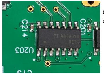
Currently on production, the Pcba with this component Fail the FVT.
