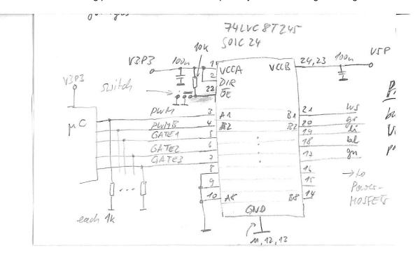
Schematic of part with latch SN74LVC8T245
