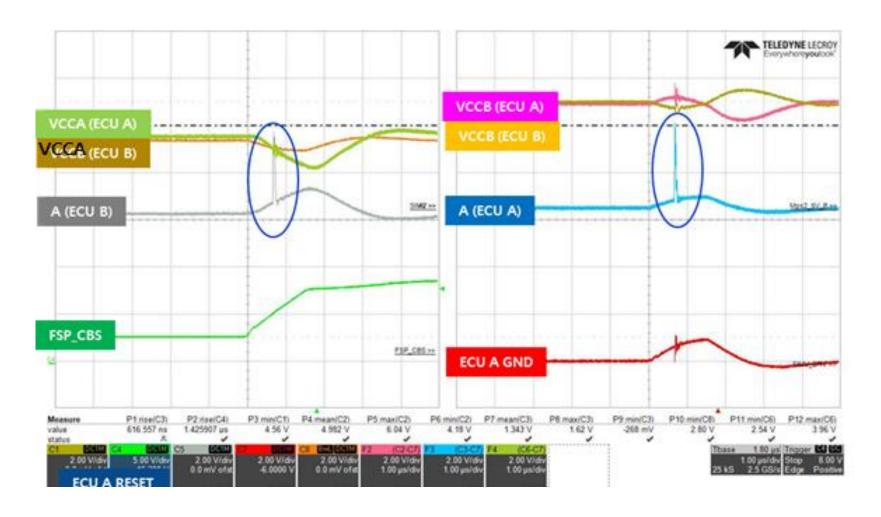
The voltage spikes are occurred on the A pin of TXS0102-Q1 on both ECU-A board and ECU-B board, respectively as above waveform.
