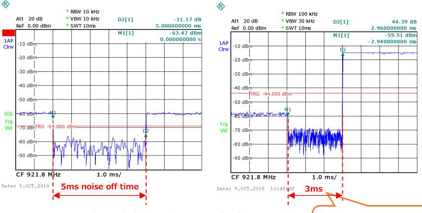
To meet Japan regulation, below conditions need to be met. Carrier sense time: 5ms, 24ch:920.6MHz to 31ch:922.0MHz Carrier sense time: 128us, 33ch:922.4MHz to 61ch:928.0MHz
