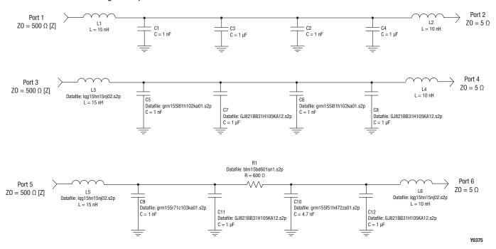
Figure 2. Circuit Diagrams with Suggested Part Numbers from Murata
