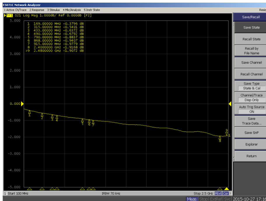
Figure 7. Insertion Loss of MXFR01JA3000 Low-Cost Cable
