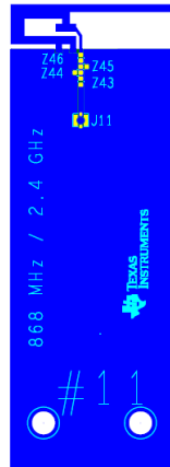
Figure 43. Board #11: 2.4 GHz PCB Antenna
