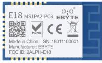
E18-MS1PA2-PCB adopts the original CC2530 RF chip of TI, the chip is integrated with 8051 MCU and wireless transceiver, and built-in PA+LNA, greatly expanding communication distance and improving communication stability. The module is applicable for ZigBee design and 2.4GHz IEEE 802.15.4 protocol.
