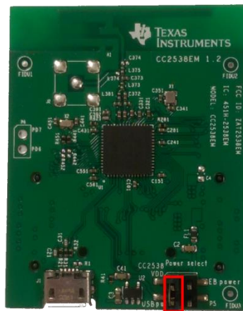
Figure 5 Jumper position for USB connection
