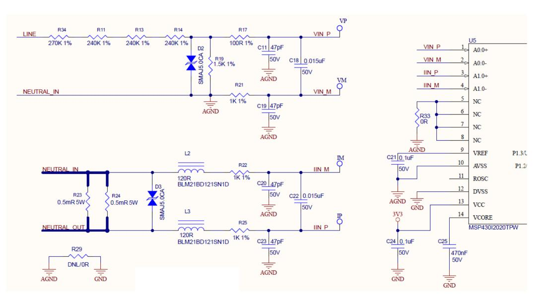
Page-2 : Power Supply Note : There is a bridge rectifier in between Neutral\_IN & GND
