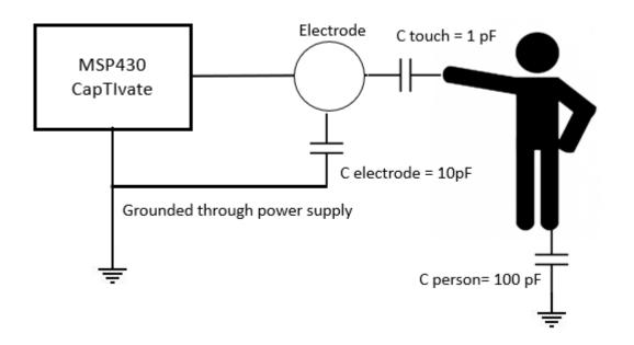
$$Sensitivity\ Line\ Powered = \frac{\frac{1}{\frac{1}{C\ touch} + \frac{1}{C\ person}}}{C\ electrode} = \frac{\frac{1}{\frac{1}{1pF} + \frac{1}{100pF}}}{10pF} = \frac{0.99pF}{10pF} = \frac{\sim 1pF}{10pF}$$
