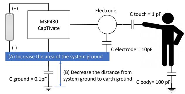
Improve system coupling to earth ground by A, B or both.
