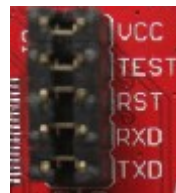
Figure 39. eZ430 Debug Connector on MSP-EXP430G2 LaunchPad
