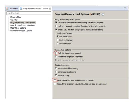
10. Unselect the check box as below red circles then "Remember My Settings", Now connect the FET with target board, be careful that we possible reset the target at this step if the connection is not stable during operation. You can try with normal target board to make sure your operation will not reset the chip before connect the hanging board.
