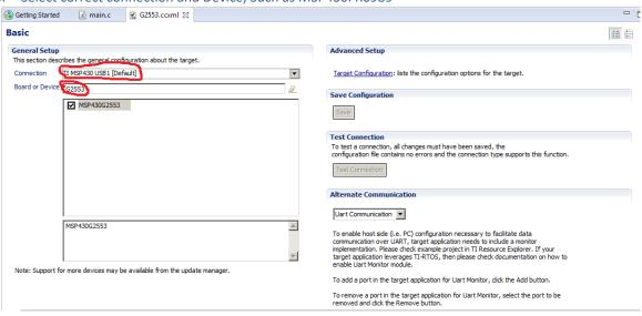
6. After "Save", there is a new ccxml file under User Defined, then connect the MSP-FET with computer, important!!! Connect FET only! not target board.
