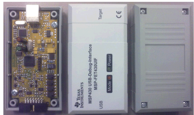
Figure 31. MSP-FET430UIF Version 1.3 Top and Bottom Views
