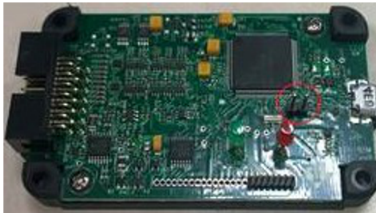
Figure 17. MSP-FET Rev 1.2 Jumper J5
