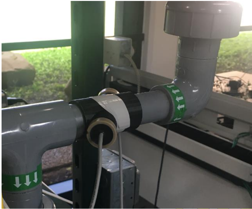
Figure 7: Flow meter test setup
