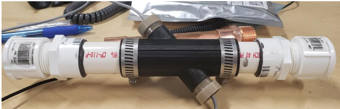
Figure 3: 3D Printed fixture attached the PVC pipe
