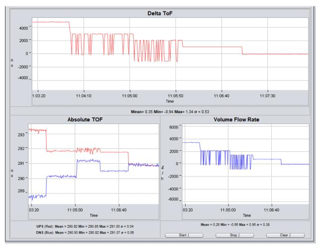
The fundamental frequency of this transducer is about 310 kHz, so the period is about 3.22us. The spikes we see in the Delta ToF chart are also very close to 3.2us, so it appears that the algorithm is getting out of phase by 1 period. Notice in the following ADC captures that the UPS and DNS are shifted by about 1 period. It appears that the algorithm is having trouble distinguishing 6 L/min from zero flow.
